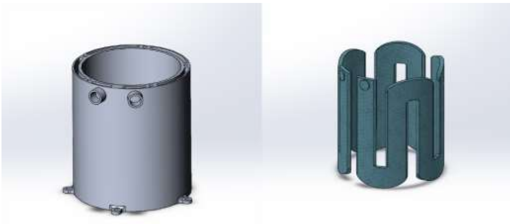
Figure 3.11 - Concept 7 Serpent circuit and water representation
