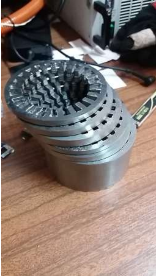
Figure 9.9 - Damaged stator parts after first attempt of insertion
