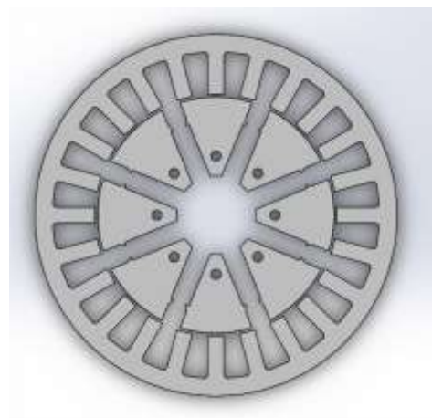
Figure 3.7 - Concept 3 stator and rotor representation
