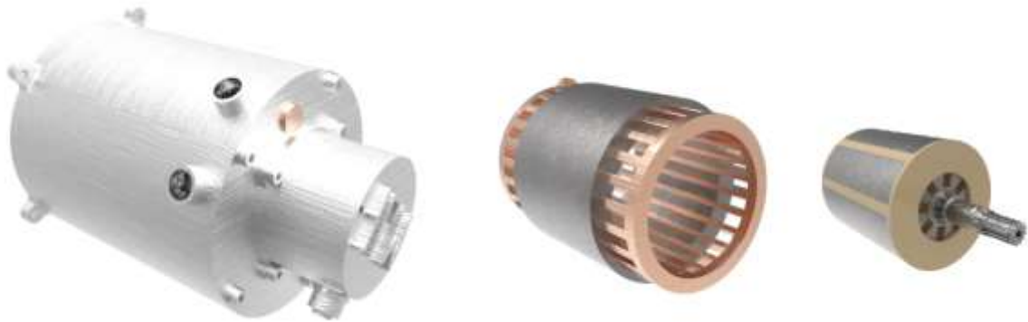
Figure 2.1 - Second Generation Motor: motor housing; stator and windings; rotor, shaft and magnets (from left to right)
