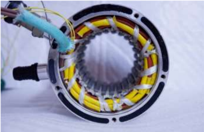
Figure 2.11 - Coils inside the stator
