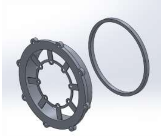
Figure 6.17 - Cooling circuit lids
