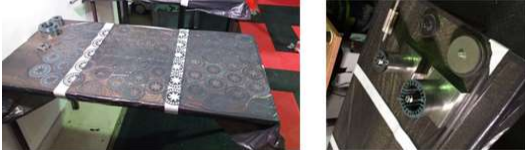
Figure 2.2 - Stator and Rotor sheets with manually applied Epoxy (left) and Stator and Rotor stacked sheets with respective JIG (right)
