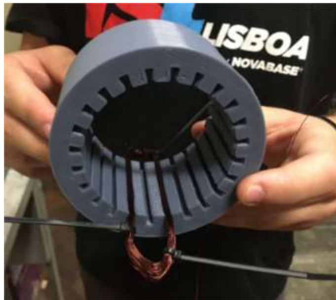
Figure 2.10 - Winding homemade attempt with 3D printed plastic stator
