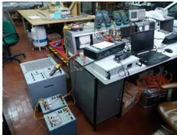
Figure 2.20 - Test-bench: capacitors, measuring devices and power supply
