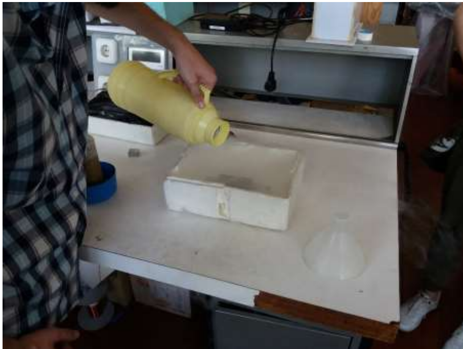
Figure 9.6 - Nitrogen application on shaft
