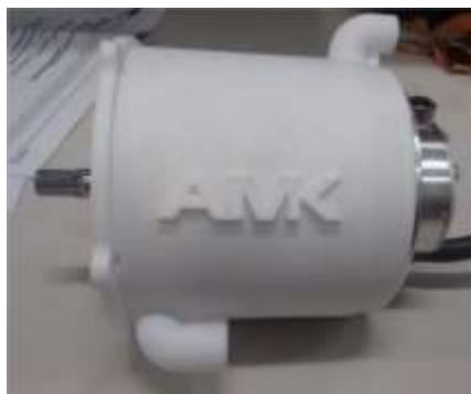
Figure 3.3 - Independent cooling housing
