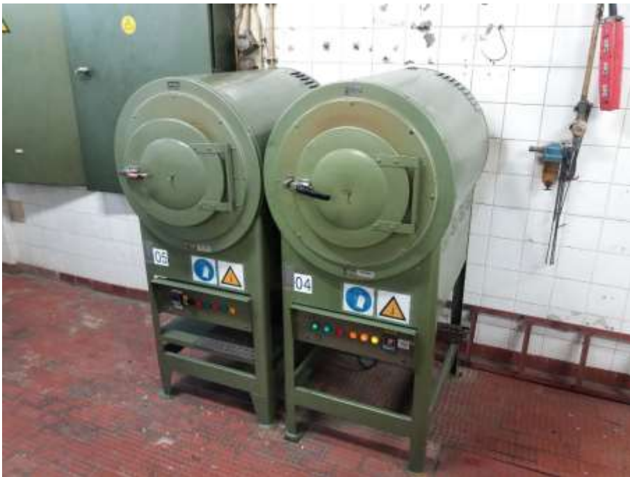
Figure 9.4 - Dry oven for epoxy cure
