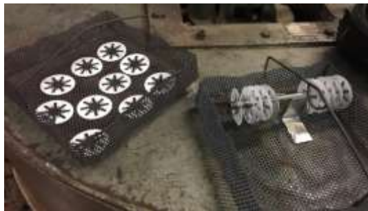
Figure 2.3 - Rotor samples drying
