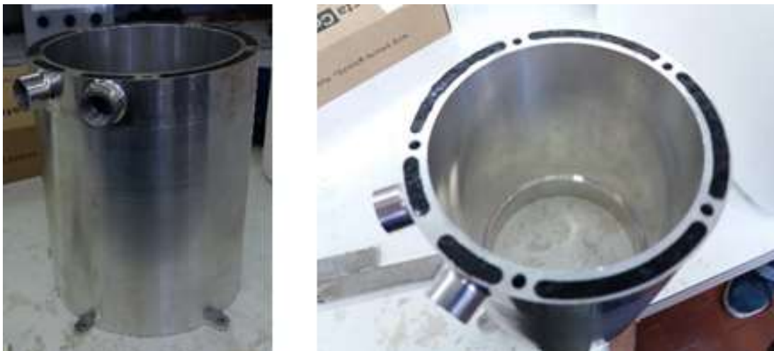
Figure 2.5 - Two view of the machined motor housing
