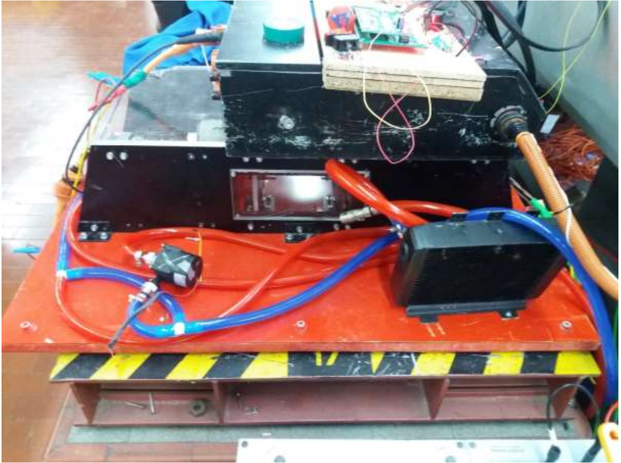
Figure 9.15 - Test bench with Invertors and cooling circuit
