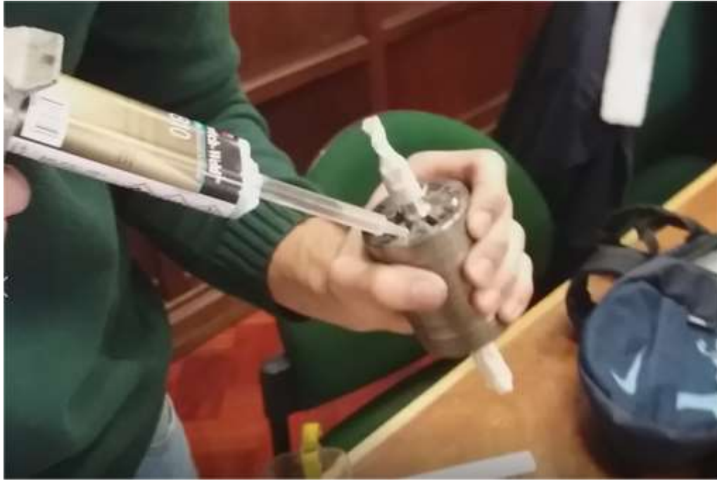
Figure 9.7 - Epoxy application for bonding magnets
